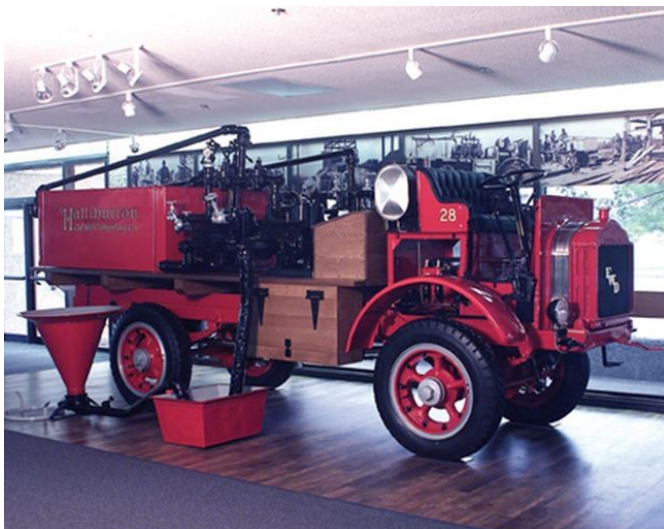
One of the earliest self-propelled Halliburton ce- menting trucks; observe the Jet Mixer at the rear of the truck on the left
